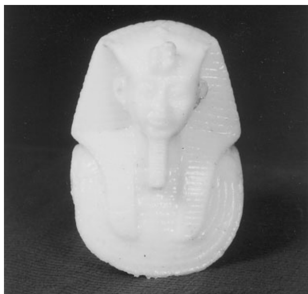
Figure 8 Death mask of Tutankhamen statue prepared from WEP1 with 20 wt % water (original magnification, 1 \times ).
