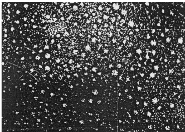
Figure 5 Microphotograph of a W/O emulsion of UP resin P1 (original magnification, 300 \times ).
