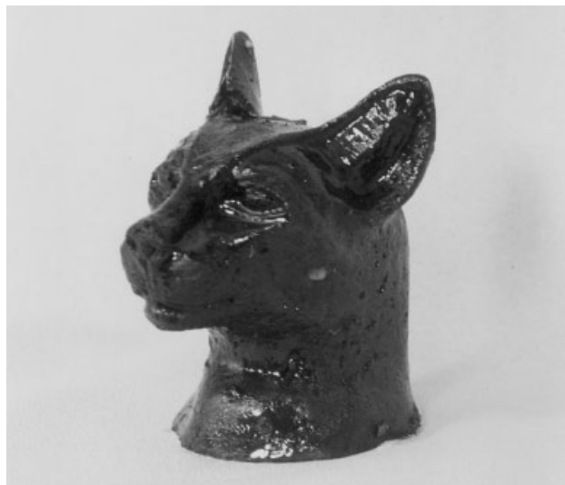
Figure 10 Black cat figurine prepared from WEPI with 40 wt % water and 6 wt % carbon black (original magnification, 1 \times ).
